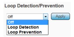
Loop Detection: the LINK/ACT LED will blink in a regular time (about 1s). Loop Prevention: One Ethernet port will be disabled and then up again.
